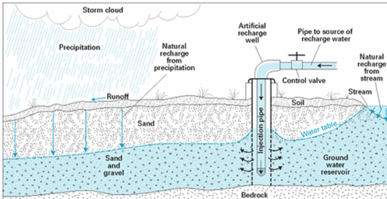
In such areas where top layer clay is impervious and its thickness is comparatively more, aquifer is 25 to 30M deeper or more, adoption of "Recharge Well Method" will be most suitable.
