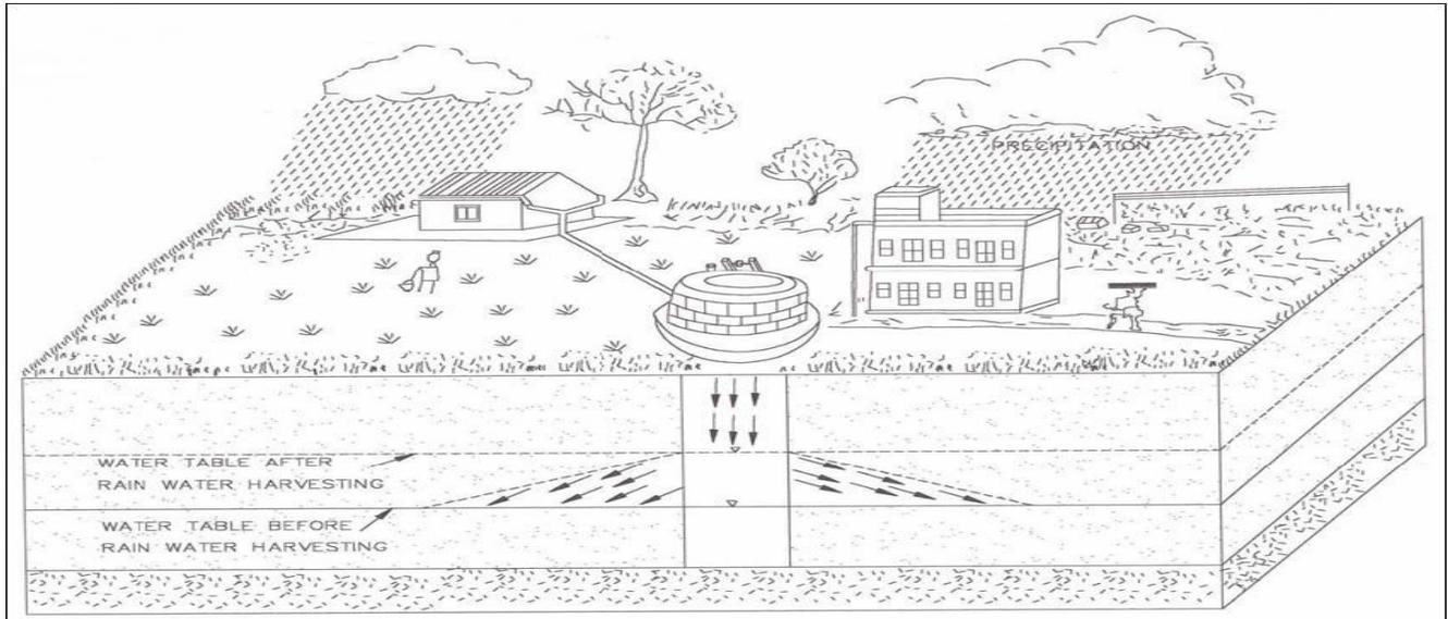
If the area of roof is 300 SQM and general rainfall is 700MM to 900MM, in this case rain water collected from rooves can be easily recharged through dry and open well.
