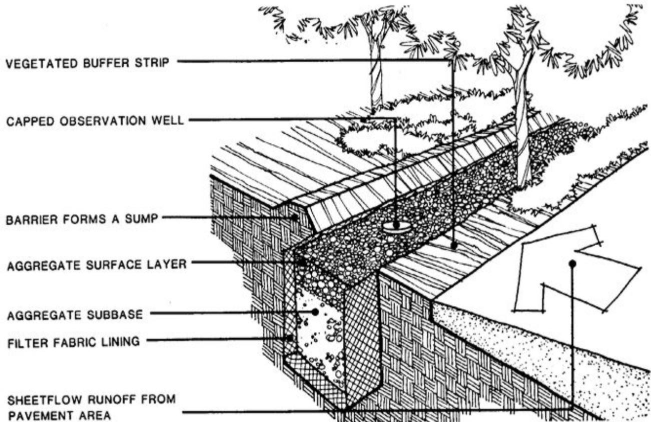
Recharge trench is also a simple method like recharge pit. Difference is only of shape and size.
