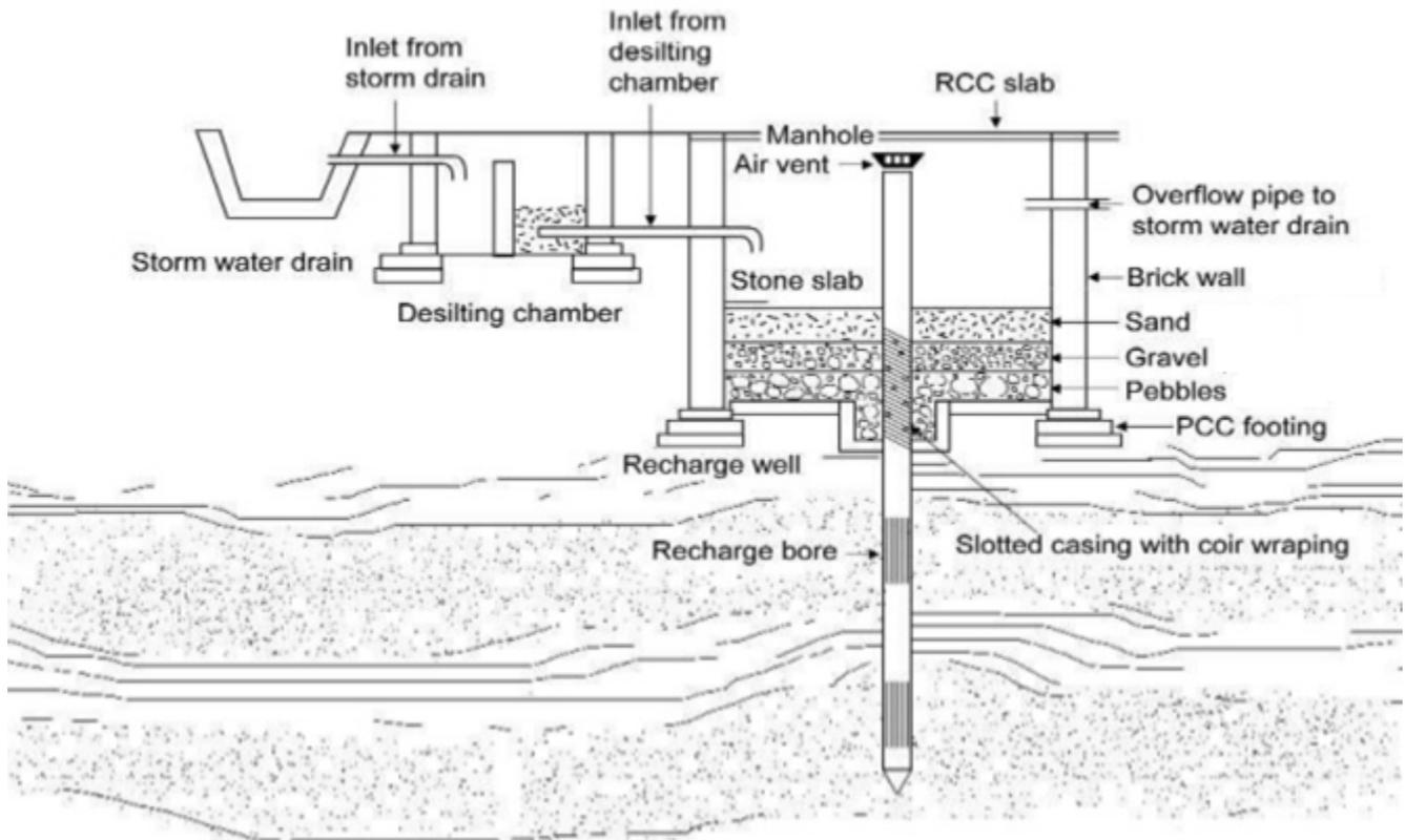
Recharge Pit Method is most suitable for such alluvial areas (plains) where permeable strata are not below than 2 to 2.5 meter deeper from the ground surface.
